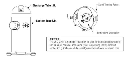
NOTE: The compressor is delivered under nitrogen gas pressure (between 4 and 6 psig). Do not disassemble bolts, plugs, fittings, etc...unless all pressure has been relieved from the compressor. Wear protective goggles and work gloves.
